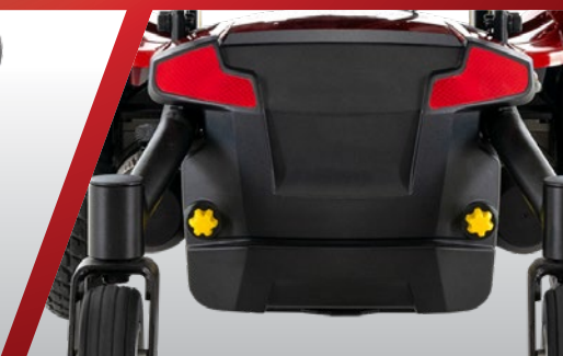
Convenient rear access to batteries
